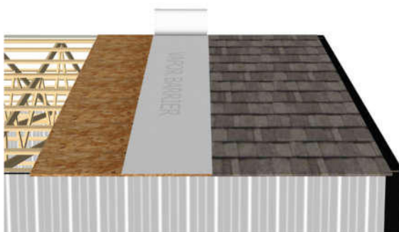
Asphalt Shingle from Owens Corning (hidden fasteners, installed over OSB)
